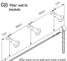
Offer track up to wall and mark a point 7cm (2³/4") in from each end. Firmly fix brackets to wall in these positions. Fix remaining brackets to wall at equal intervals between these brackets (approx. 60cm/2'0" a part) ensuring that they are perfectly level.
