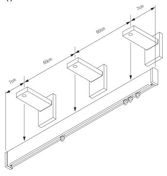
Offer track up to wall and mark a point 7cm (2³/4") in from each end. Firmly fix brackets to wall in these positions. Fix remaining brackets to wall at equal intervals between these brackets (approx. 60cm/2'0" apart) ensuring that they are perfectly level.
