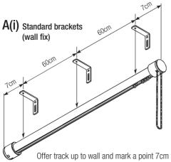
(23/4") in from each end. Firmly fix brackets to wall in these positions. Fix remaining brackets to wall at equal intervals between these brackets (approx. 60cm/2'0") ensuring that they are perfectly level.
