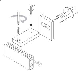
The track inserts move freely inside the top channel of the track: line them up with each bracket, starting at each end, and screw down into the insert through the bracket until tight.
